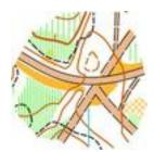
Snippet of the ISSOM map showing how the asphalt roller ski trail is mapped with solid black edge line while naturalsurfaced trails have dashed edges..
